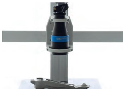
TCSM imaging and measuring sloped objects
